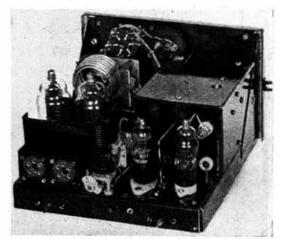
This rear view of the transmitter shows the general layout. All components for the Clapp oscillator with the exception of the cathode choke and resistance are housed in the screening box on the right. The plate condenser for the TTI1 buffer stage can be seen to the left of the valve and is controlled from the panel by means of an extension spindle.
