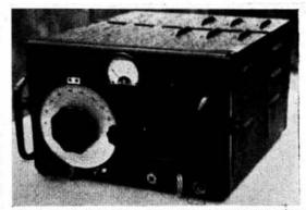
The transmitter is housed in a well-louvred case measuring 11 in. x 7 in. x 11½ in. The V.F.O. dial is inscribed 0-180° and can be conveniently calibrated by graph and abac.
